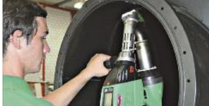
Even inside radiuses are easy to weld.
