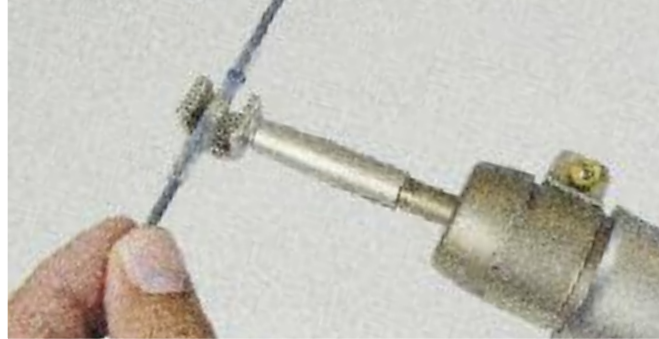
TRIAC AT shrinking a cable connection.
