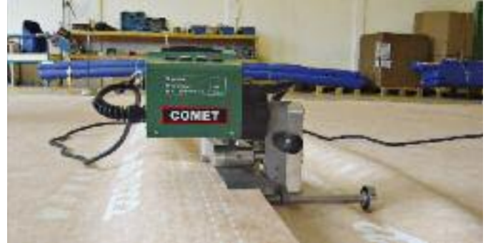
Hands-free welding due to integrated guiding plates.
