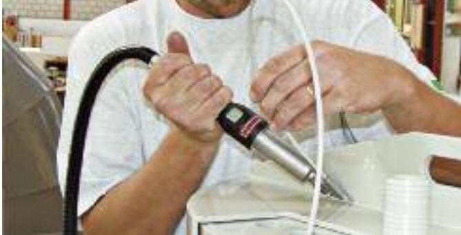
Draw welding using the compact and lightweight WELDING PEN R.
