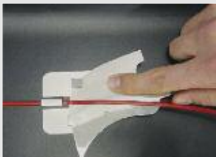
Step 3: Pulling out the inserted welding rod with trimmer and spatula. (page 34)
