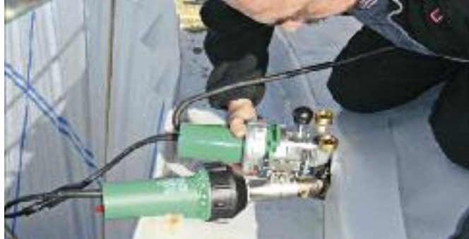
The TRIAC DRIVE PID allows even horizontal welding.
